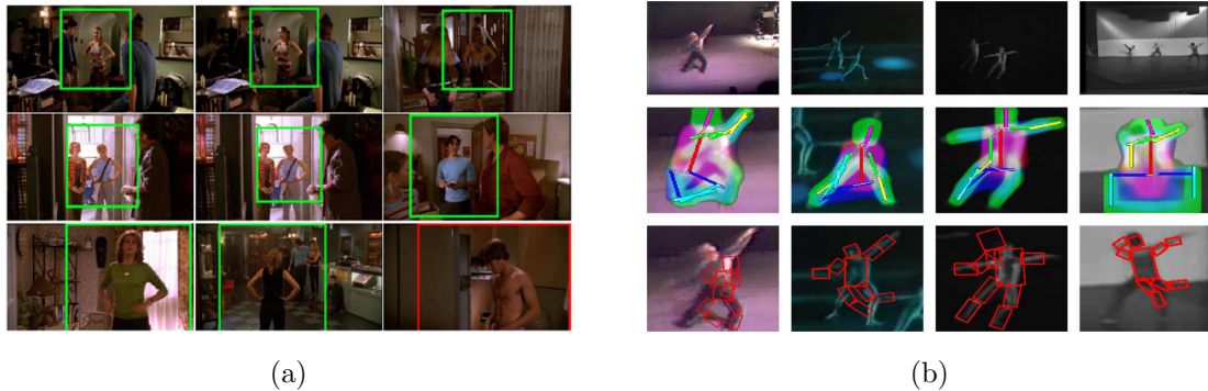
Figure 2.11 (a) Using upper-body human pose estimation for retrieval [74] where the top left is the query and the top 9 results.(b) Challenges of human pose estimation making it currently unsuitable for retrieval showing: top – original frame, middle – approach of Ferrari et al. [73], bottom – approach of Yang et al. [235]. Where figures are from respective publications.
